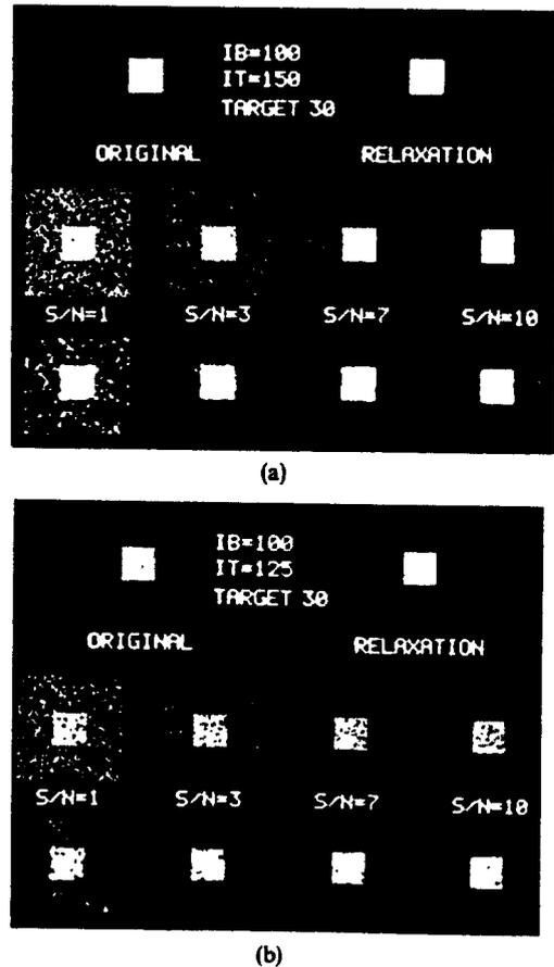
Fig. 4. Effect of contrast and noise on target extraction. (a) Target size  $30 \times 30$ , target intensity 150, background intensity 100. (b) Target size  $30 \times 30$ , target intensity 125, background intensity 100.
