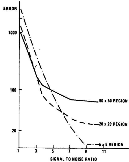
Fig. 3. Pixel classification error vs signal-to-noise ratio for the images in Fig. 2.
