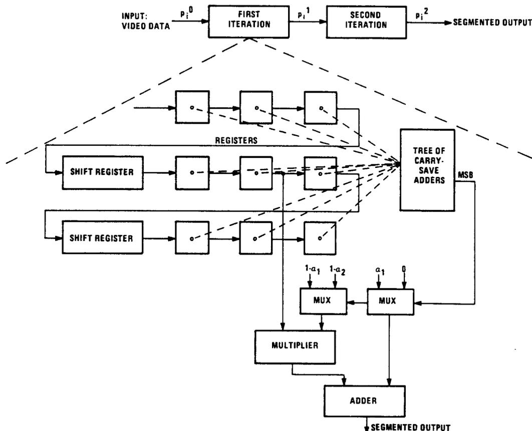
Fig. 6. Real-time implementation of the two-class gradient relaxation algorithm.
