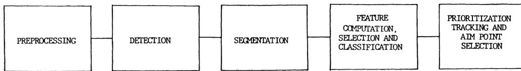
Fig. 2. Basic block diagram of typical ATR system.
