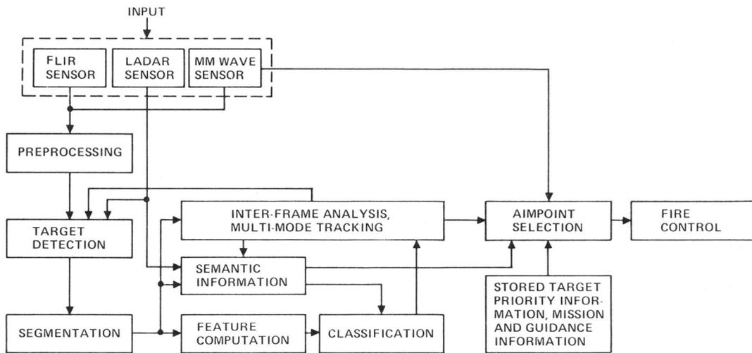
Fig. 6. Schematic diagram of multisensor ATR system.
