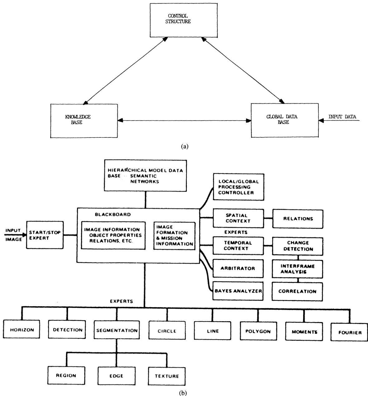
Fig. 4. K-B approach for ATR. (a) Basic structure of K-B approach. (b) Block diagram of target recognition expert system.
