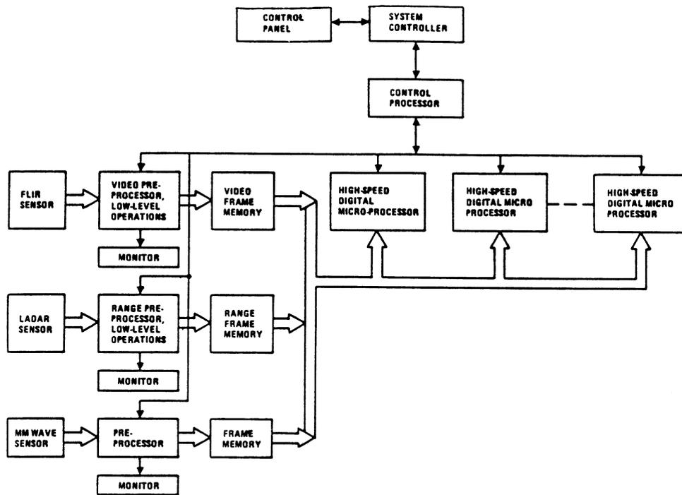
Fig. 12. Architecture of multisensor ATR system.
