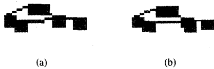
Figure 6. Polygonal approximation of the car. (a) default M2 parameter (b) learned M2 parameter.
