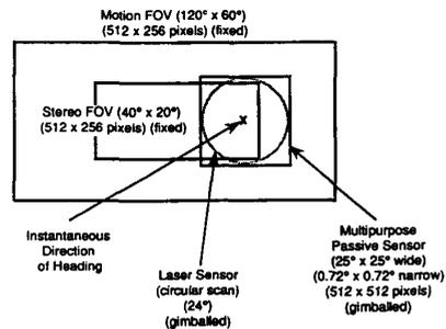
Figure 2: Overlapping fields-of-view for the ODIN system.
