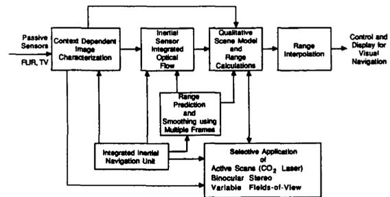
Figure 1: The schematic diagram of the ODIN system.
