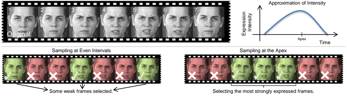
Fig. 4: Comparison of sampling at even intervals versus sampling at the apex. A video is given, and its expression intensity is given. Sampling at even intervals retains frames that are further away from the apex. They are weakly expressed, and they are not a good representation of the emotion being expressed. Sampling at the apex retains the frames where the emotion is most strongly expressed.
