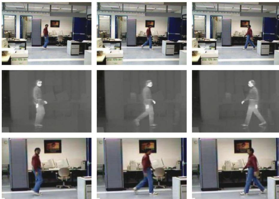
Fig. 8. Examples of registration results: first row—original color images, second row—original thermal images, third row—transformed color images.
