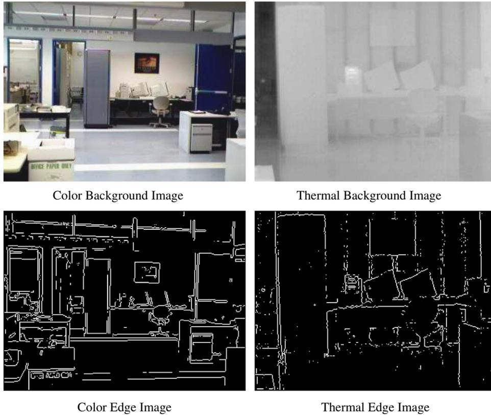
Fig. 4. Different object appearances in color and thermal images are due to the phenomenological differences between the image formation process of EO and IR cameras. The images are at different resolutions and the field-of-views (FOVs) of the two cameras overlap (EO camera FOV contains IR camera FOV).
