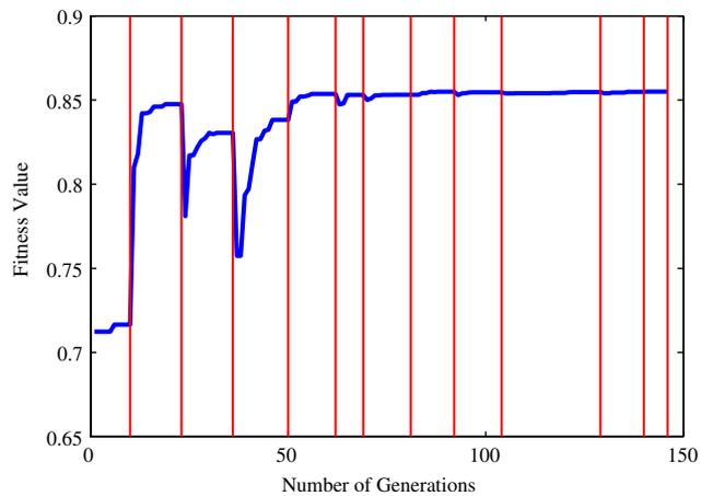
Fig. 12. Variation of fitness values from good initial correspondence. The vertical line corresponds to the last generation at each search level. The curve between two adjacent vertical lines indicates the variation of GA fitness values at a search level.
