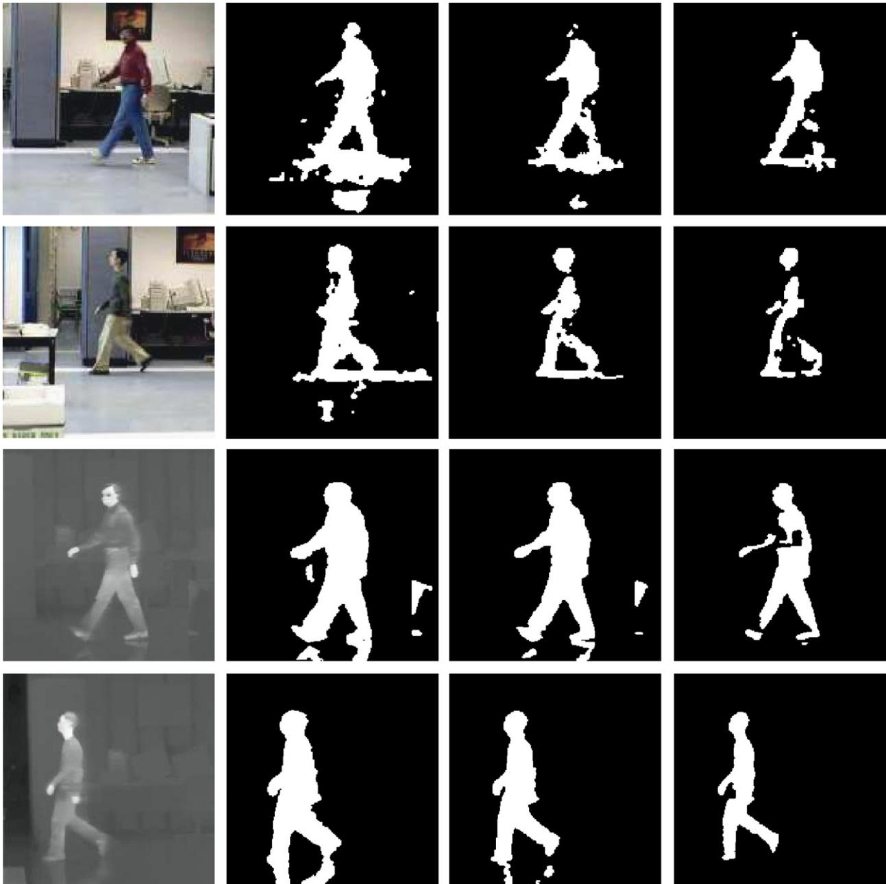
Fig. 1. Human silhouette extraction results from color images (first two rows) and thermal images (last two rows) using the background subtraction method with increasing thresholds from left to right. The leftmost image is the original image.
