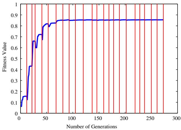
Fig. 11. Variation of fitness values from bad initial correspondence. The vertical line corresponds to the last generation at each search level. The curve between two adjacent vertical lines indicates the variation of GA fitness values at a search level.
