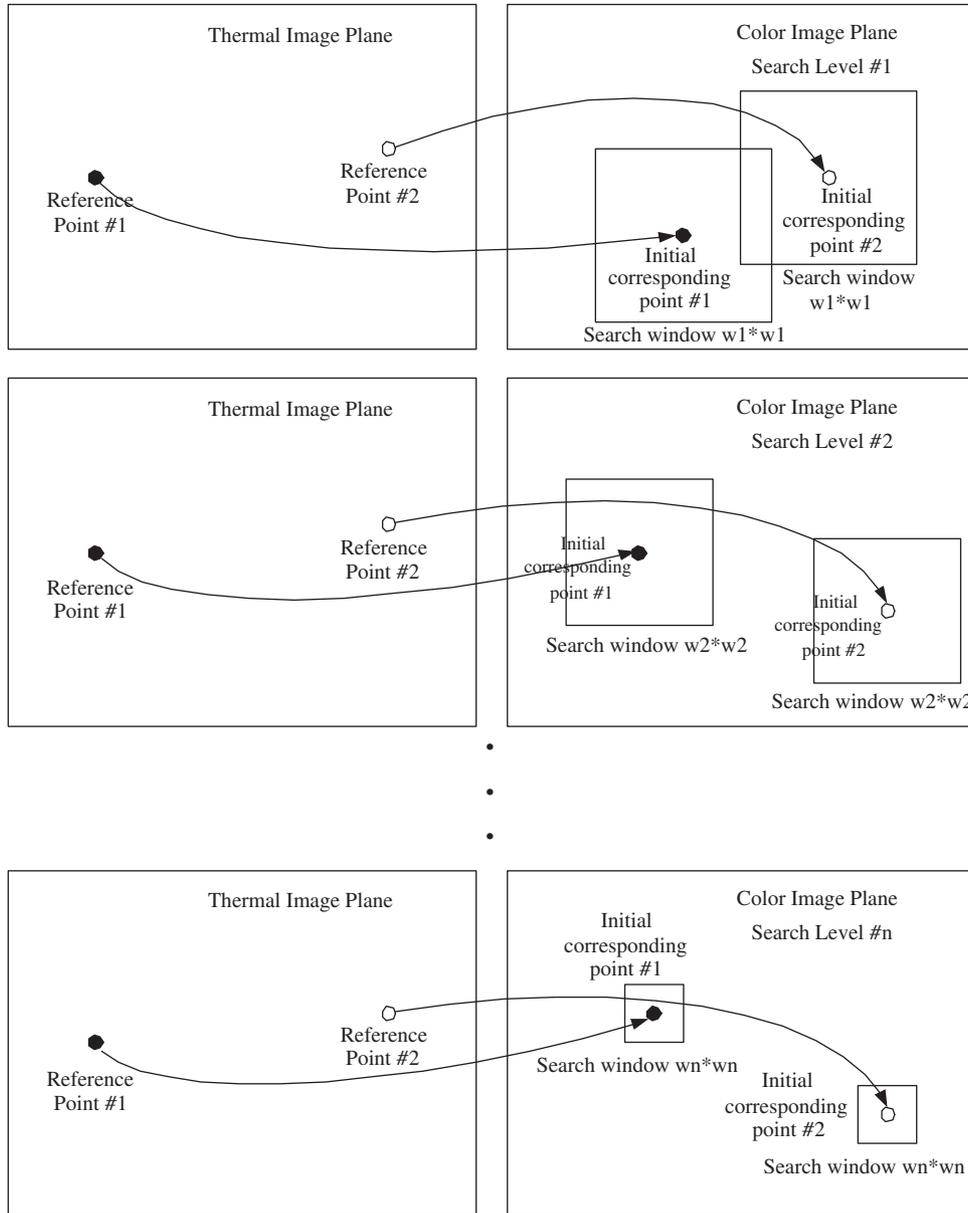
Fig. 6. Illustration of the HGA-based search scheme to estimate the model parameters—coordinate values of the two points (black and white) simultaneously in the color image plane. The search windows here are only for illustration whose sizes are much larger than the real window sizes.
