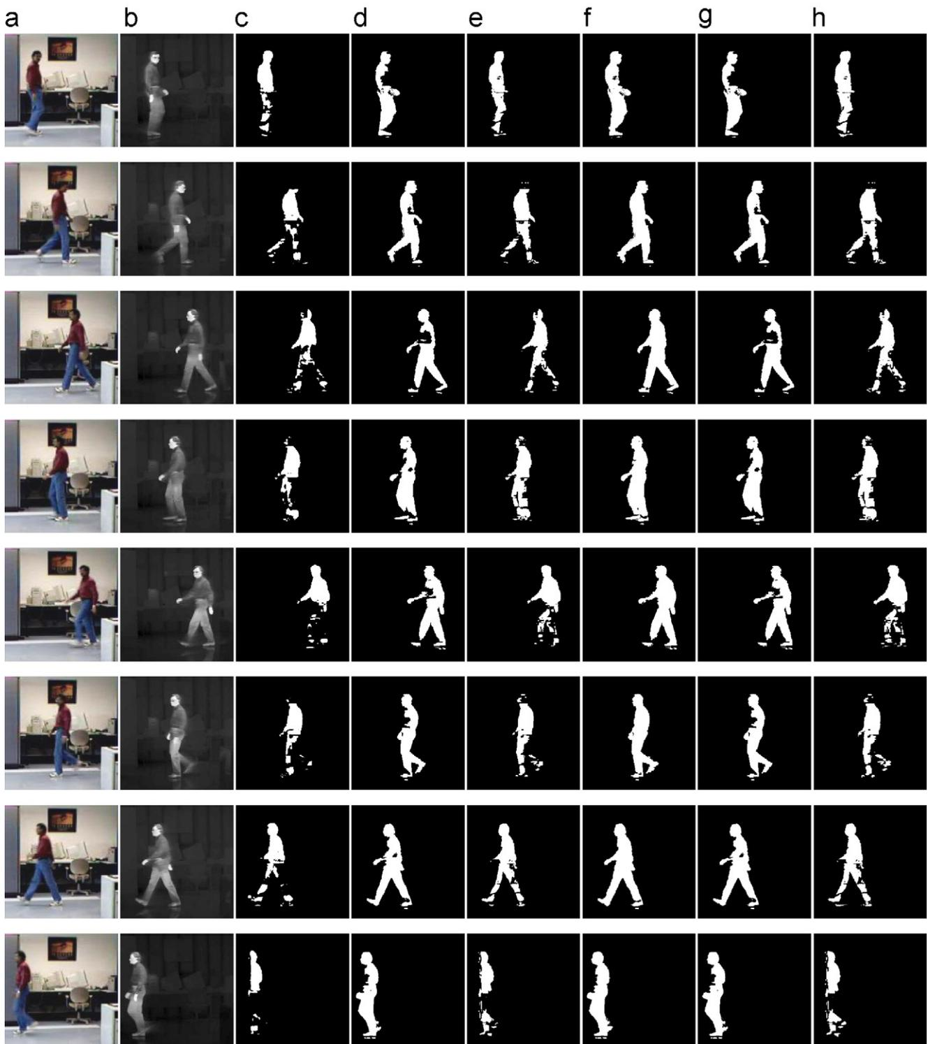
Fig. 14. Examples of fusion results: (a) transformed color images, (b) original thermal images, (c) silhouette from (a), (d) silhouette from (b), (e) silhouette from product rule fusion, (f) silhouette from sum rule fusion, (g) silhouette from max rule fusion, (h) silhouette from min rule fusion.
