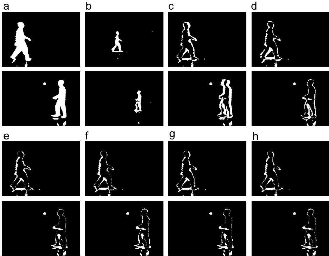
Fig. 9. Examples of estimated transformation results from good initial correspondence: (a) original silhouettes from thermal images, (b) original silhouettes from color images, (c) matching error of the initial transformation, (d) matching error after the first search level, (e) after the second search level, (f) after the third search level, (g) after the fourth search level, (h) after the 12th search level.
