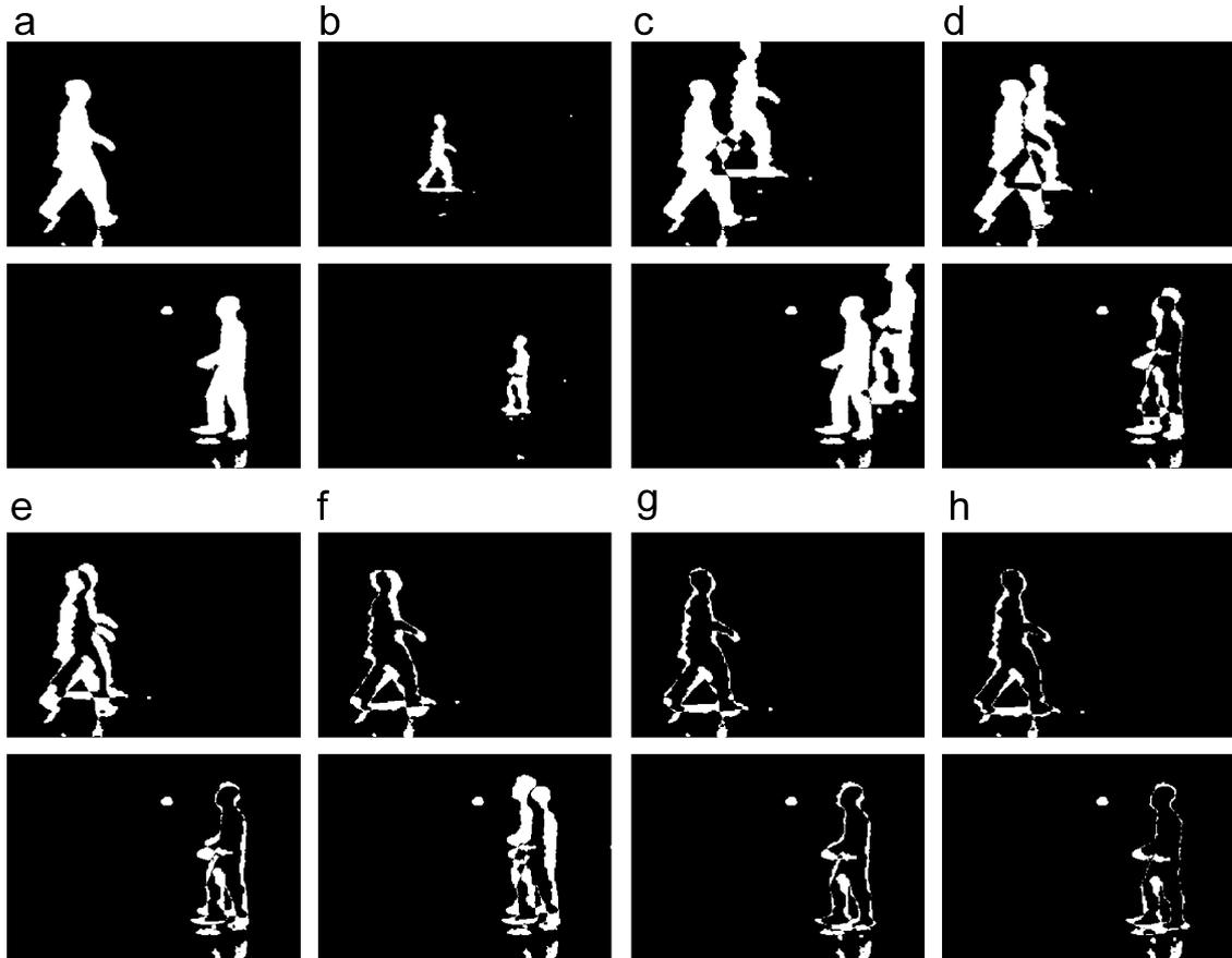
Fig. 10. Examples of estimated transformation results from bad initial correspondence: (a) original silhouettes from thermal images, (b) original silhouettes from color images, (c) matching error of the initial transformation, (d) matching error after the first search level, (e) after the second search level, (f) after the third search level, (g) after the fourth search level, (h) after the 23th search level.
