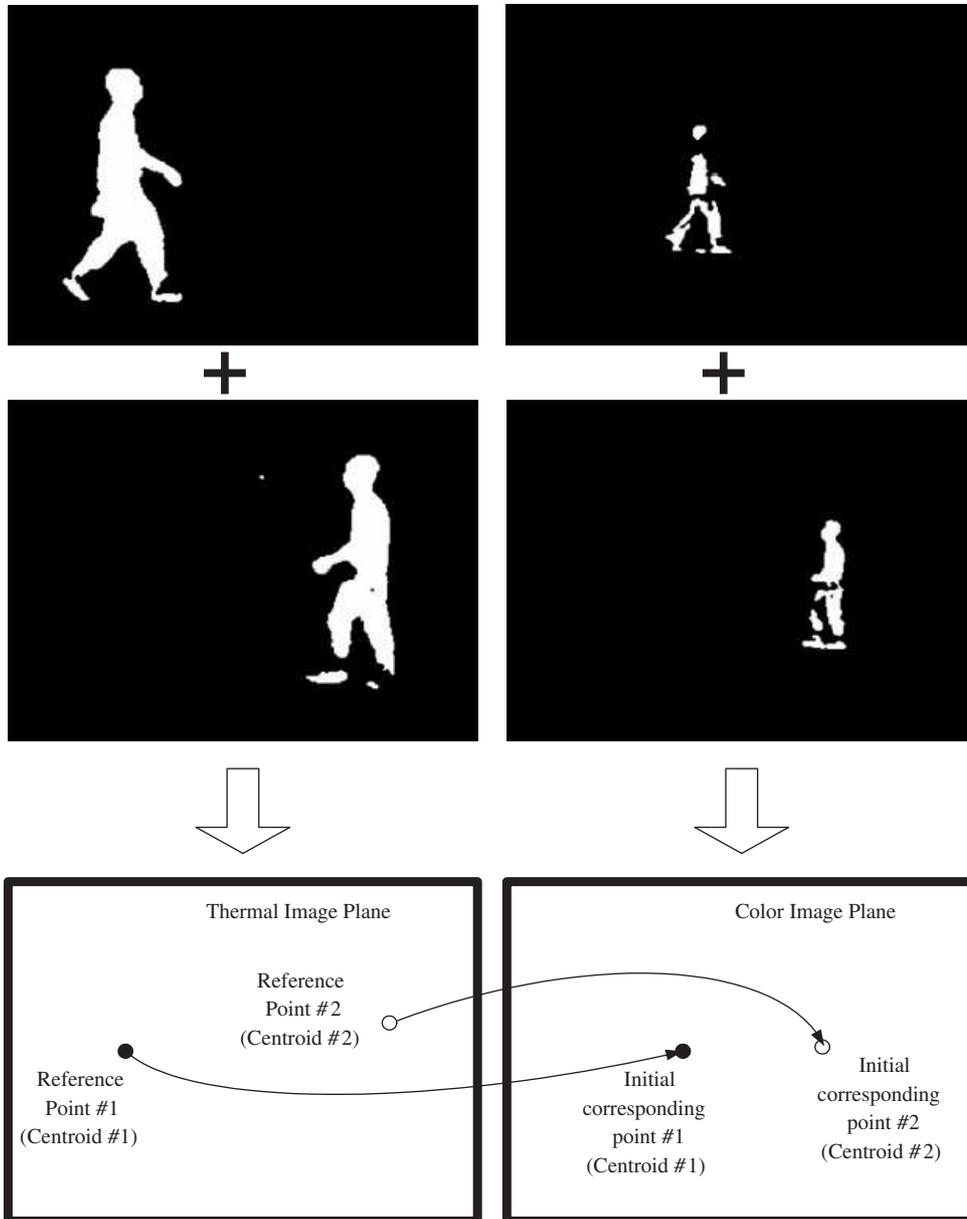
Fig. 5. Illustration of initial control point selection in both color and thermal image planes.
