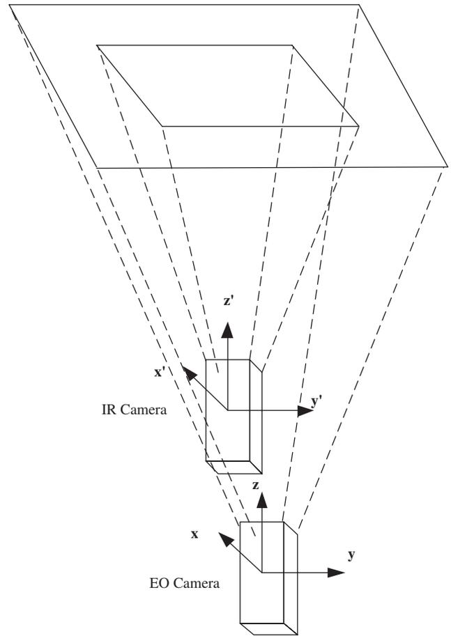
Fig. 3. IR and EO camera set-up.
