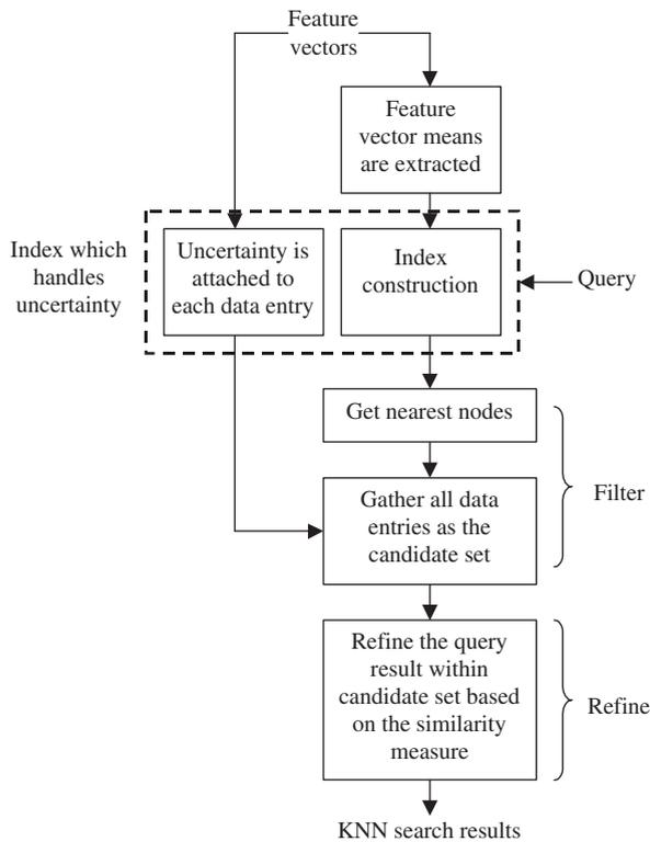
Fig. 2. System diagram for uncertainty handling spatial database.
