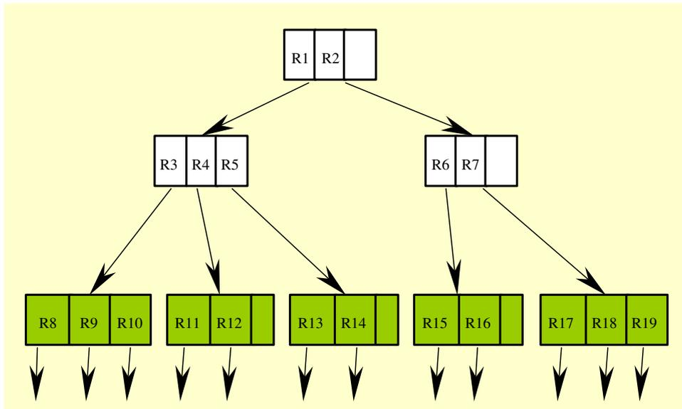
Fig. 6. R-tree structure of Fig. 5.
