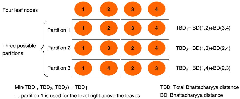
Fig. 4. Tree construction—agglomeration algorithm.
