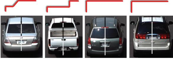
**Figure 1: Top: Canonical structure, Bottom: Rear views (Black line: parallel to the road; White line: almost perpendicular to the road)**
