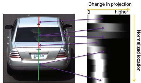
Figure 5: Structural signature occurrences for sedans (Right: Brighter means more frequent; darker means less frequent)
