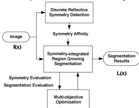
Fig 1. System diagram for symmetry integrated segmentation.
