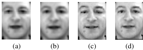
Figure 4. Comparison of reconstruction results on semi-synthetic data. (a) Low-resolution image. (b) Bi-cubic interpolated image. (c) Uniformly reconstructed image. (d) Non-uniformly reconstructed image.
