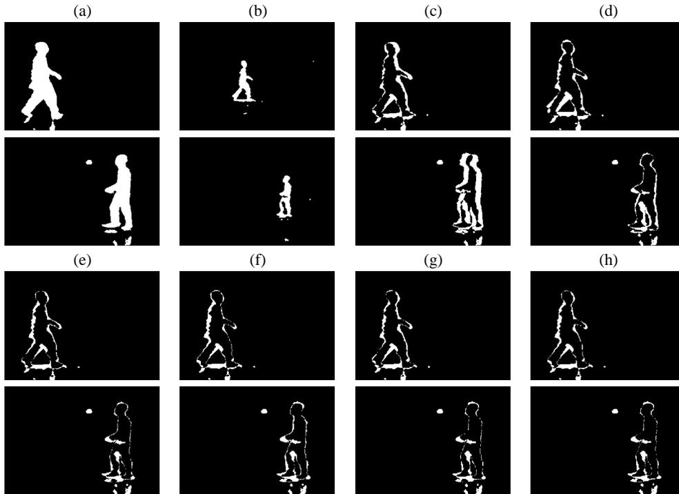
Figure 5: Example of estimated transformation results from good initial correspondence: (a) original silhouettes from thermal images, (b) original silhouettes from color images, (c) matching error of the initial transformation, (d) matching error after the first search level, (e) after the second search level, (f) after the third search level, (g) after the fourth search level, (h) after the 12th search level.
