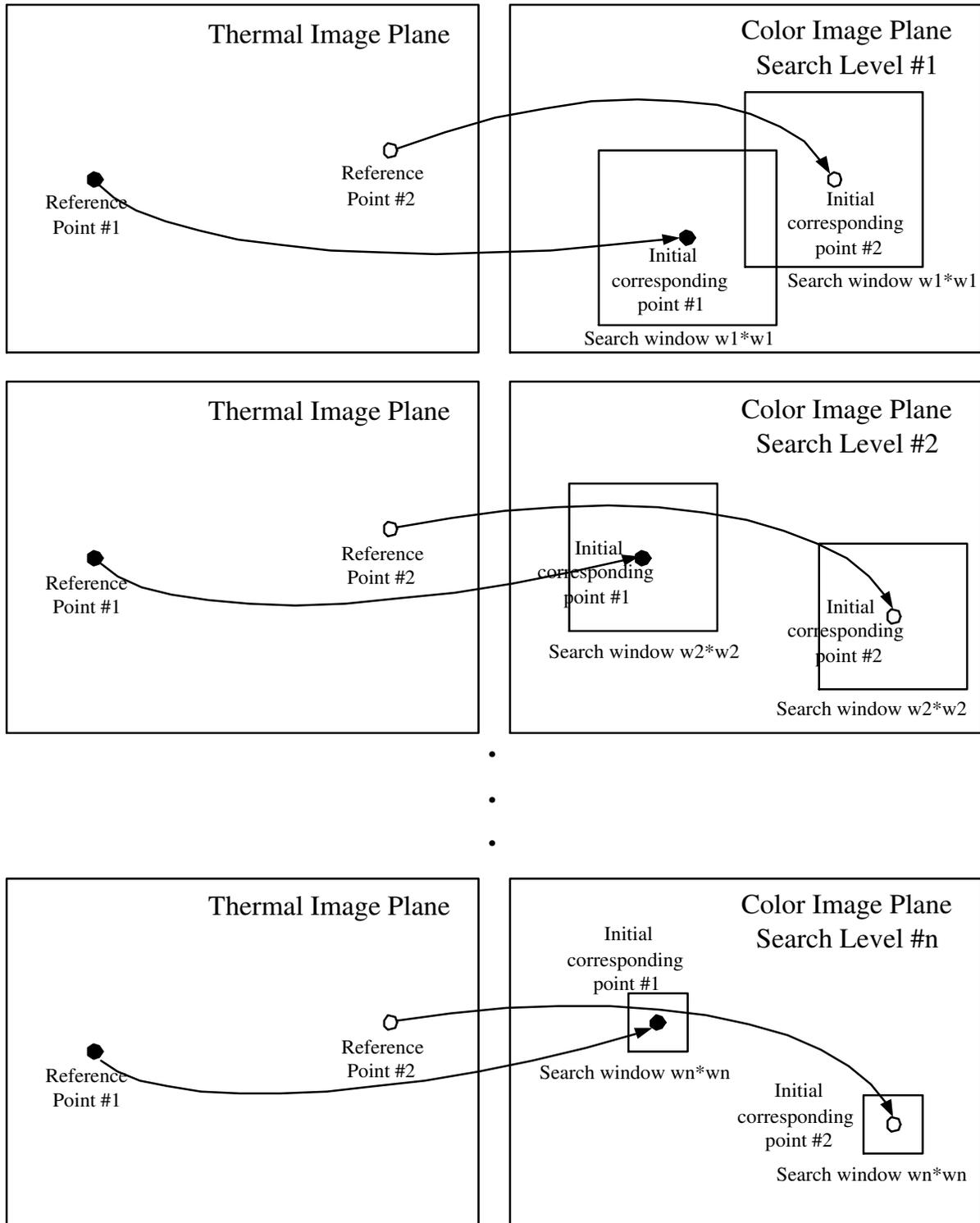
Figure 3: HGA-based search scheme to estimate the two 2-D point locations (black and white) simultaneously in color images. This graph only illustrates the procedure of correspondence estimation. The search windows here are only for illustration whose sizes are much larger than the real window sizes.
