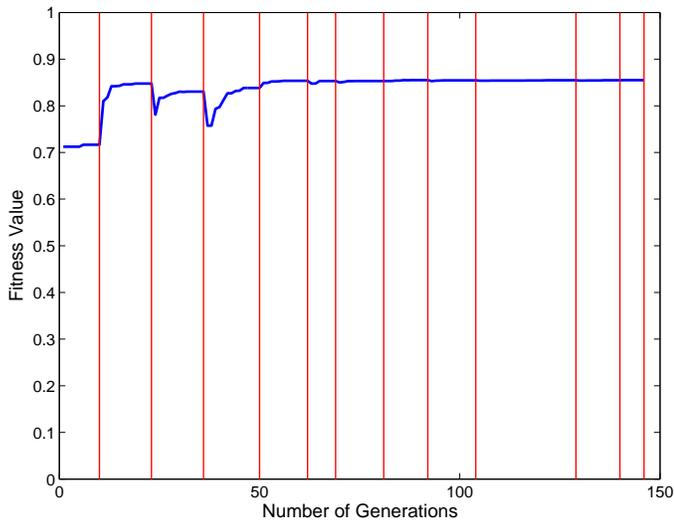
**Figure 7: Variation of fitness values from good initial correspondence. The vertical line corresponds to the last generation at each search level. The curve between two adjacent vertical lines indicate the variation of GA fitness values at a search level.**
