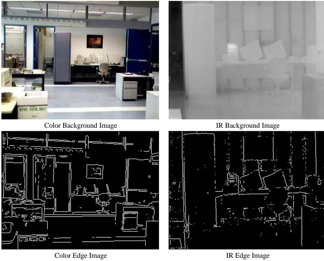
**Figure 2: Different object appearances in color and IR images are due to the phenomenological differences between the image formation process of color and IR video sensors. The images are at different resolutions and the field-of-views (FOVs) of the two sensors overlap (Color video sensor FOV contains IR video sensor FOV).**
