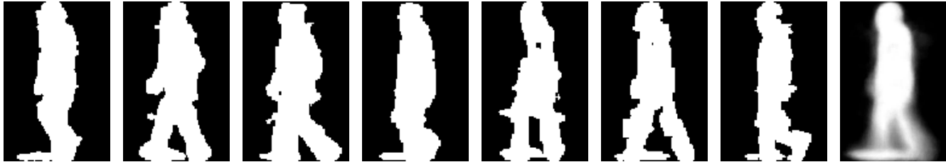
Figure 1. Examples of normalized and aligned silhouette frames in a human walking sequence. The rightmost image is the average silhouette image over the whole sequence - Gait Energy Image (GEI).
