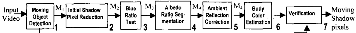
Figure 1. Different steps of physics-based shadow detection algorithm. M_i is the binary Mask of potential shadow pixels updated after each step.
