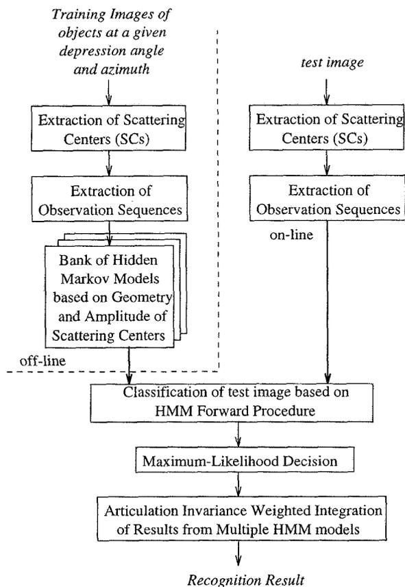
Figure 1: The HMM-Based approach for recognition of articulated objects.
