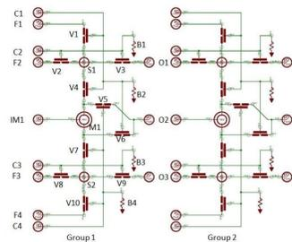
Microfluidic Schematic Built from Symbolic Components
